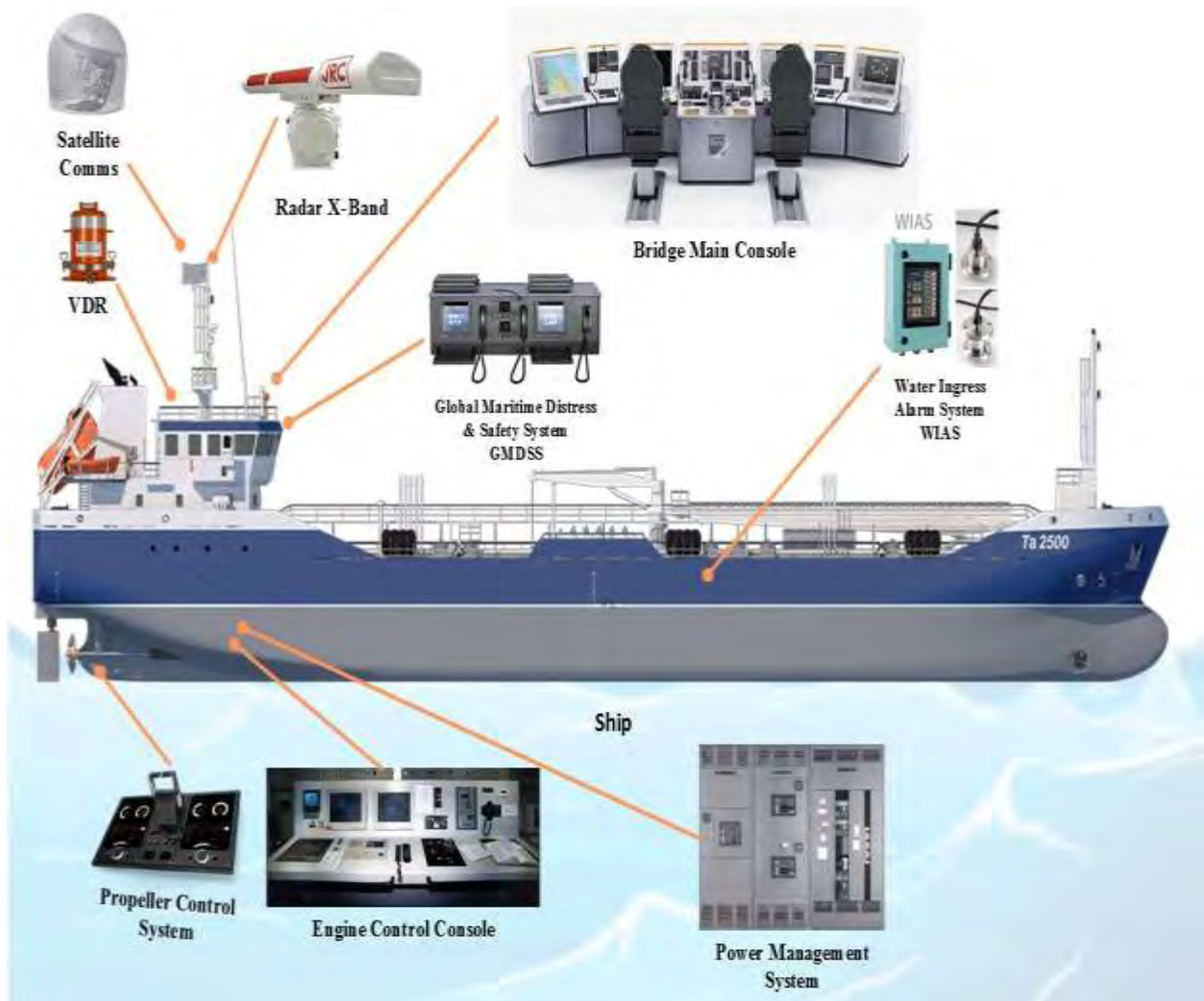
Picture 4 Vessel's Operation Technology Systems (OT)
