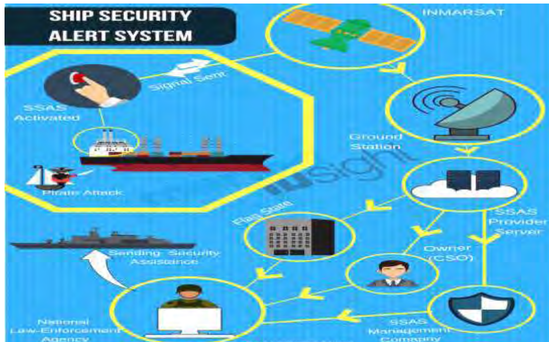
Picture 23 Shipboard Security Alarm Systems (SSAS)
