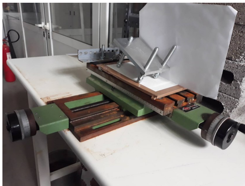
Figure 2.3: milling machine table with the moving saddle
