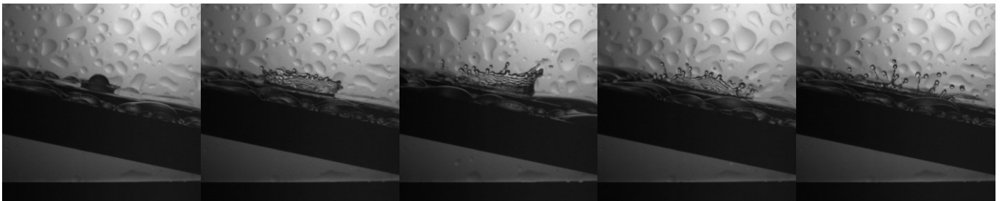
Figure 3.7: Evolution of droplet impingement for \theta=10^\circ , We=260 , Ra=6.99\mu\text{m}
