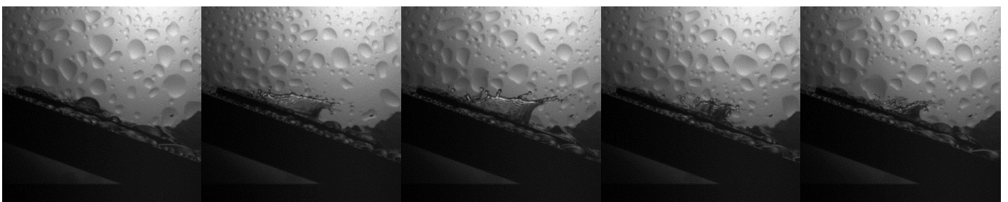
Figure 3.13: Evolution of droplet impingement for \theta=20^\circ , We=260 , Ra=1.37\mu\text{m}
