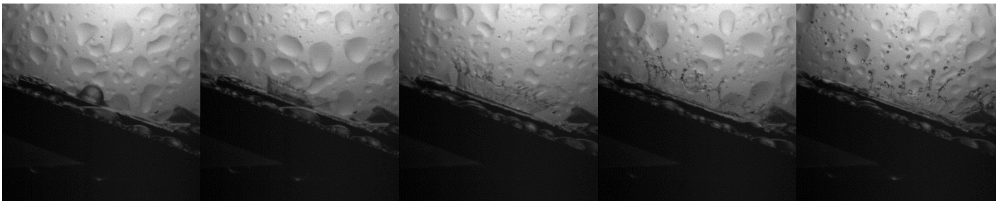
Figure 3.12: Evolution of droplet impingement for \theta=20^\circ , We=534 , Ra=0.06\mu\text{m}
