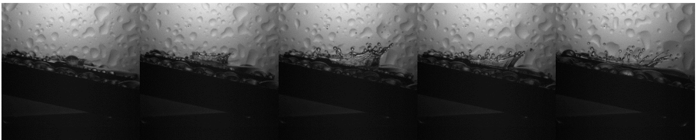
Figure 3.1: Evolution of droplet impingement for \theta=10^\circ , We=260 , Ra=0.06\mu\text{m}
