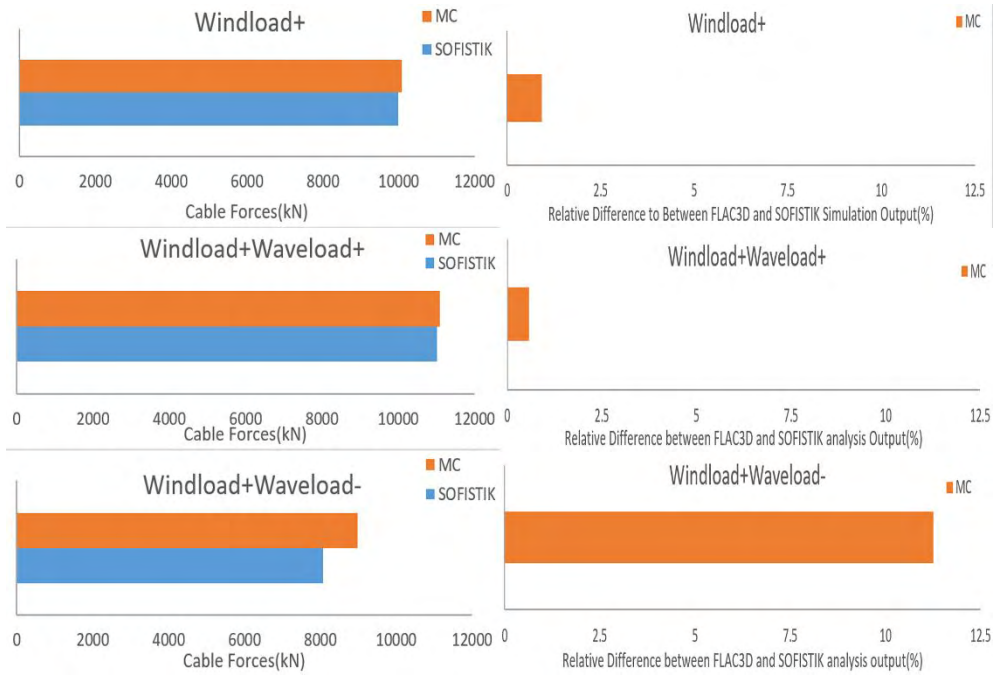
Figure C. 7 STDM and FTDM Simulation differences in terms of -xcable axial force.
