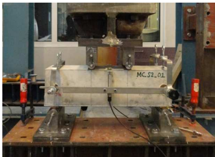
Fig. 9. Experimental setup for the 4-point bending tests: (a) schematic of the testing setup and (b) photo for size S2 beam specimen.
