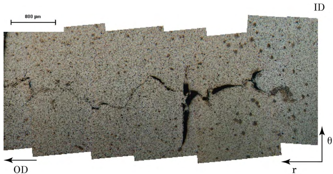
Figure 29. SOHIC at location 500.
