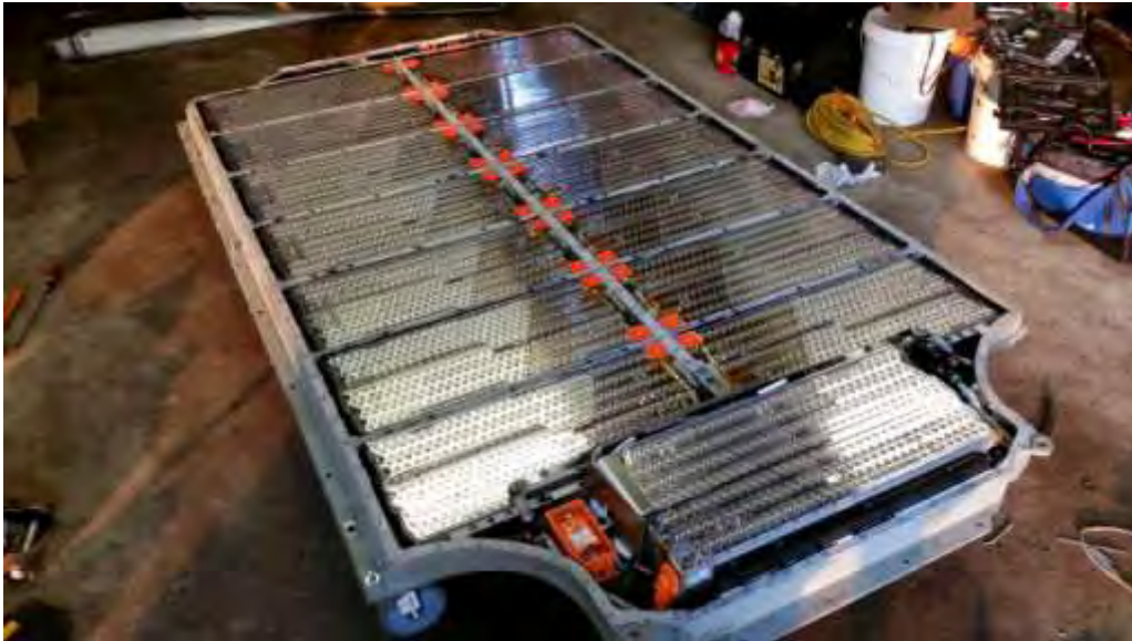
Figure 2.11: Battery pack of a Tesla Model S electric vehicle.
