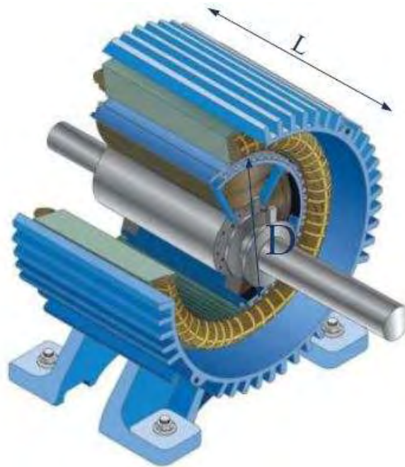
Figure 3.19: An electrical machine in which can be distinguished both the active length (L) and the diameter of the air gap (D)
