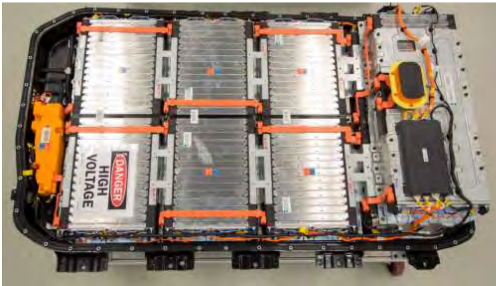
Figure 2.12: Complete Storage System of Batteries of General Motor electric vehicle
