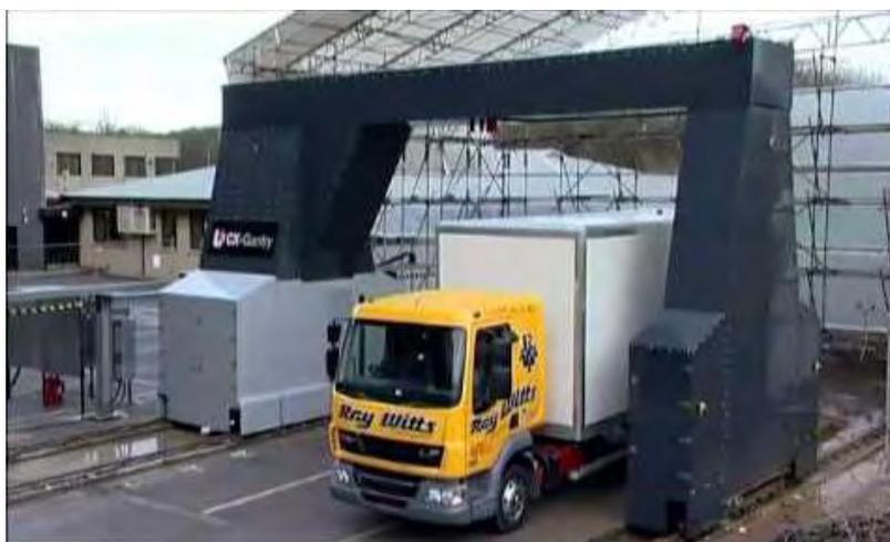
Figure 27: Heavy Cargo X-Ray Screening System
