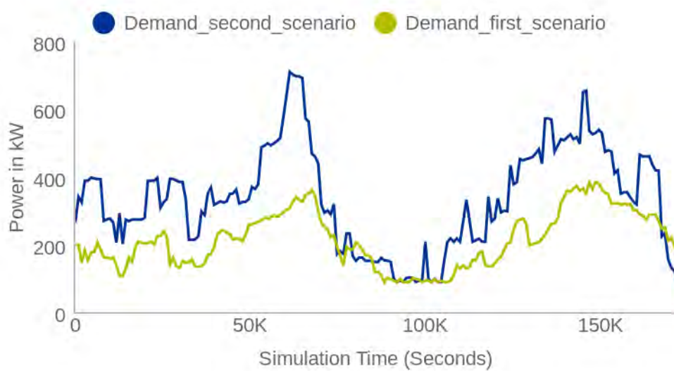
FIGURE 6.10: Demand for the residential and agricultural load for both first and second scenario with the 10 fields for two days simulation.
