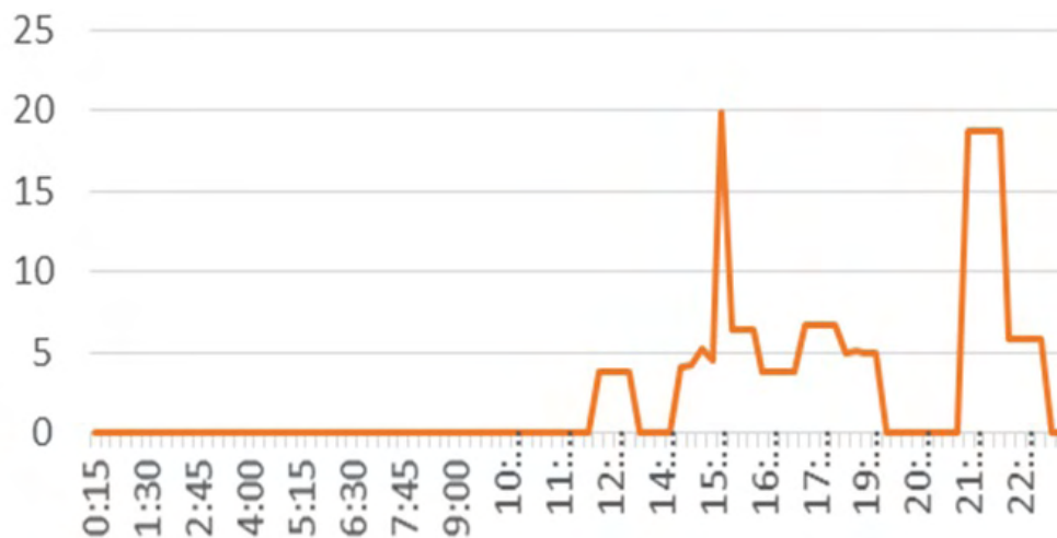
FIGURE 4.1: Clearing quantity of the global market of the first market model. The y-axis corresponds to the power in MW and the x-axis to the simulation time.
