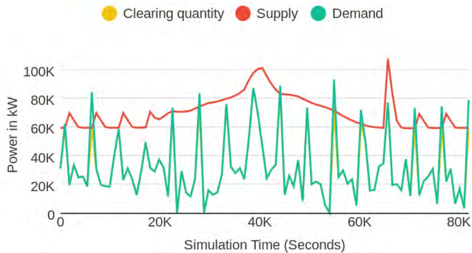
FIGURE 6.2: Market Clearing: The demand, supply and clearing quantity in kW correspond to y axis while the x axis represents the simulation time which is 24 hours for the first scenario with one field.
