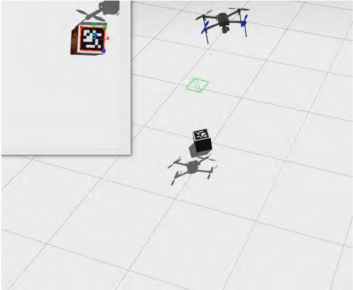
Figure 5.9: Meanwhile the Drone starts rotating (change it's heading - nose of the quadcopter) in order to align its axes with the marker's one.
