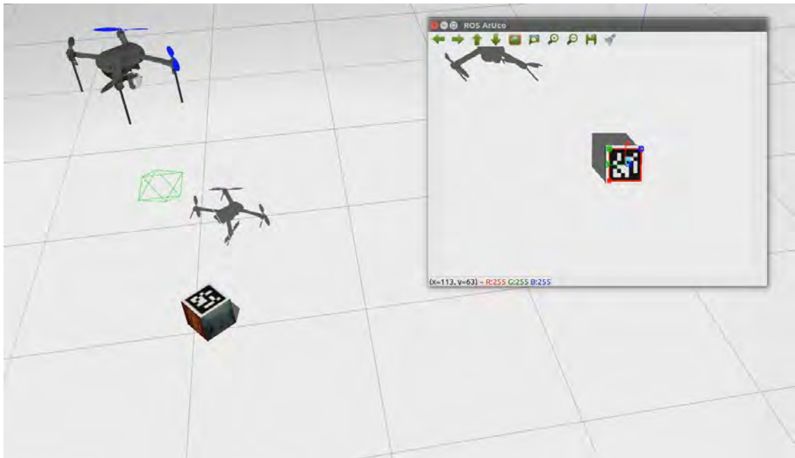
Figure 5.10: Illustration of the Drone's position and orientation after the completion of the translation and rotation commands. Note that the Drone decreases its altitude at the half of its initial altitude.
