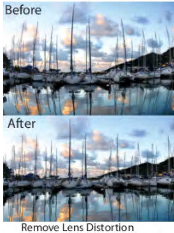
Figure 3.5: Upper image before the camera calibration procedure. Here, straight lines are seen curved because of distortion of the lens. Down image after the camera calibration procedure and correction of the lens distortion.
