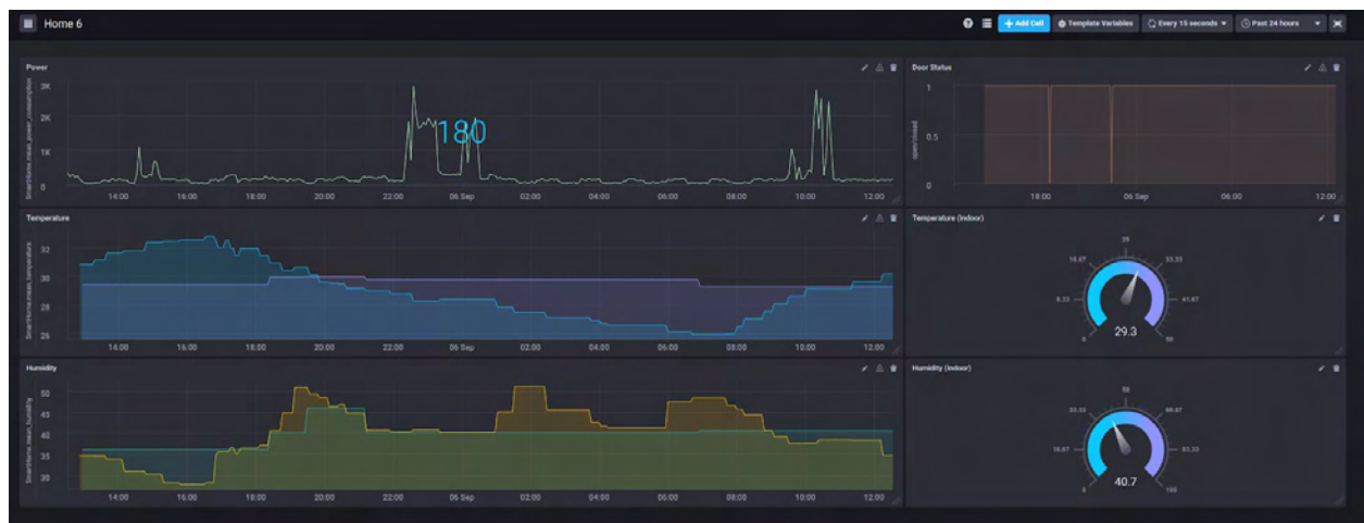
Fig. 7 power/humidity/temperature and door status for a home
