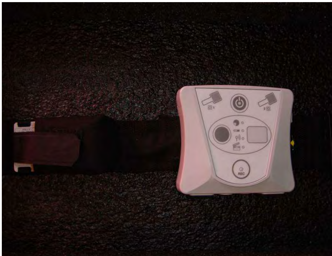
Figure 2 F-Scan ® in-shoe plantar pressure analysis with a data logger
