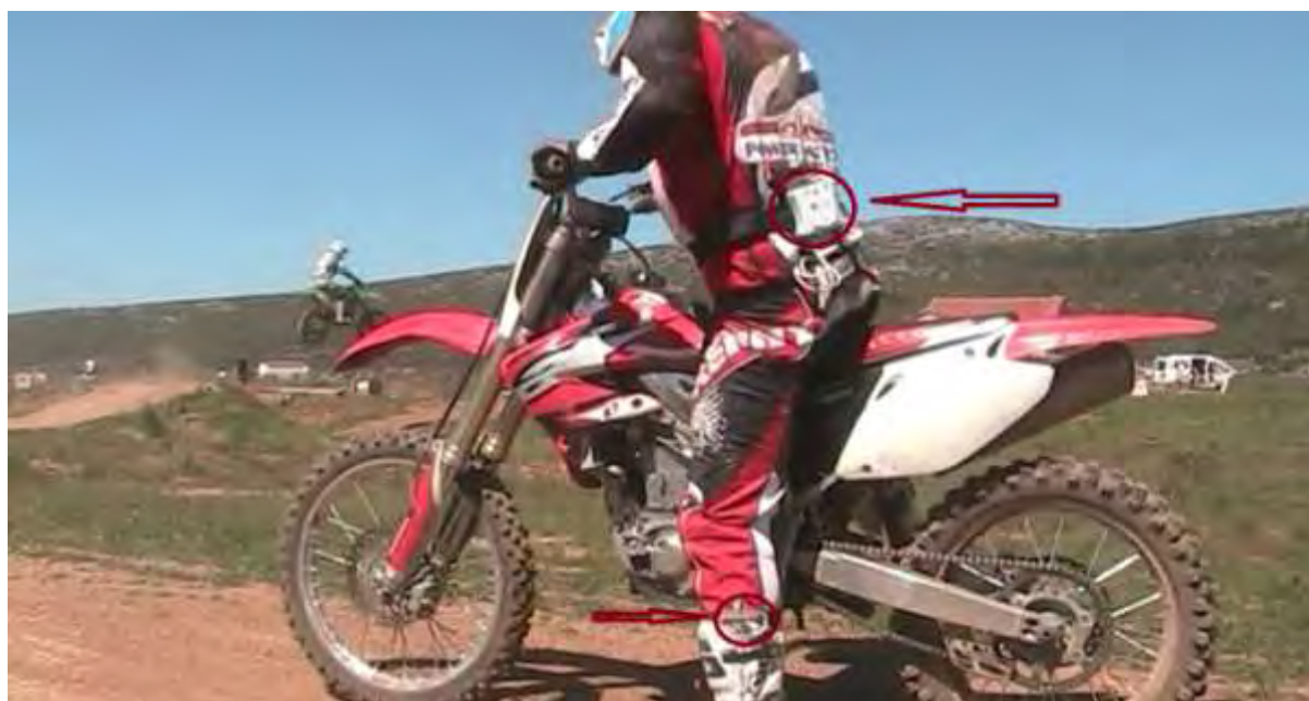
Figure 3 The data-logger adjusted on the rider during the process
