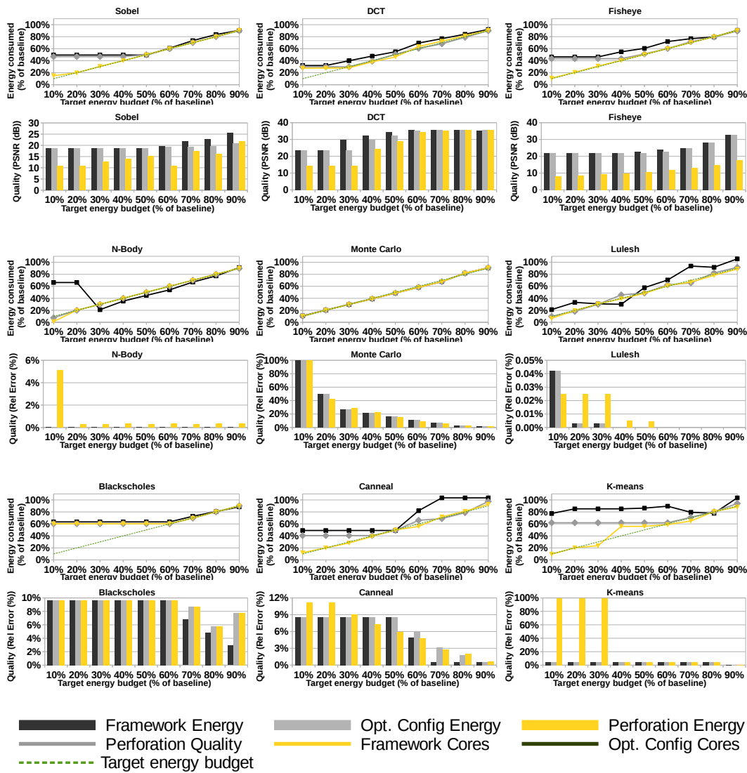
FIGURE 5.1: Quality and energy metrics for different energy targets (as a percentage of the most energy-efficient accurate execution). Energy & quality plots show the results achieved by our system, an oracle selecting the optimal configuration and loop perforation.
