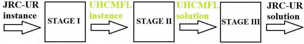
FIGURE 3.4: Our algorithms operate in three stages: In Stage I, the MNO transforms the JRC-UR into the UHCMFL instance. In Stage II, it solves that instance by employing one of the algorithms in Table 3.1. In Stage III, it maps the obtained solution to a solution for the JRC-UR instance based on the rules in Section 3.3
