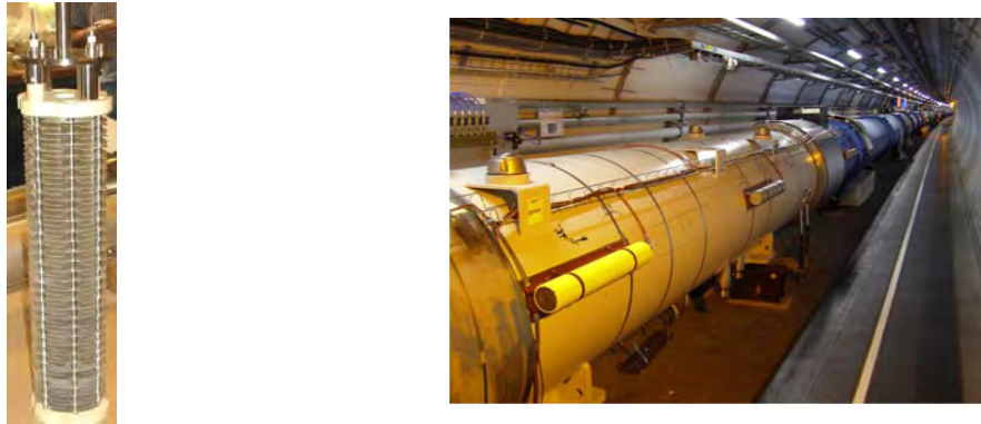
Figure 2.3: The Ionization Chambers used for the LHC Beam Loss Monitor system and their position in the quadrupole magnets of the arc [6].
