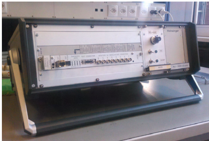
Figure 5.4: The front panel of the portable BLEDP stand-alone data acquisition system. Image courtesy of Christos Zamantzas.
