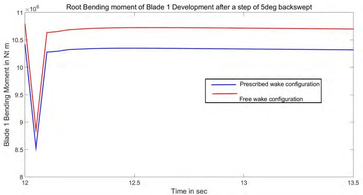
Figure 5.16 : Blade No1 Root Bending Moment Response of PW and FW code after a 5 deg backsweep step (12 sec convergence)
