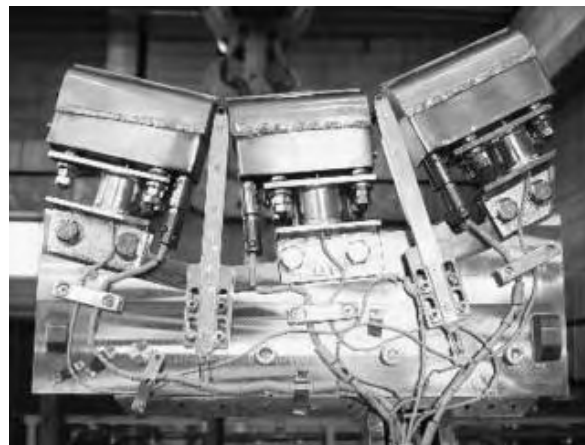
Fig. 1.9 View of complete assembled LLL before installation in FTU, [17]
