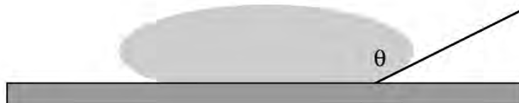
Fig. 2.1 Nonwetting case: contact angle is bigger than 90^\circ
