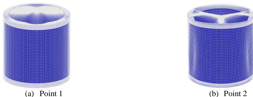
Figure 6-15: The deformed shape of the cylindrical tank at characteristic levels of temperature for the slender roof case ( t_r = t_c ).
