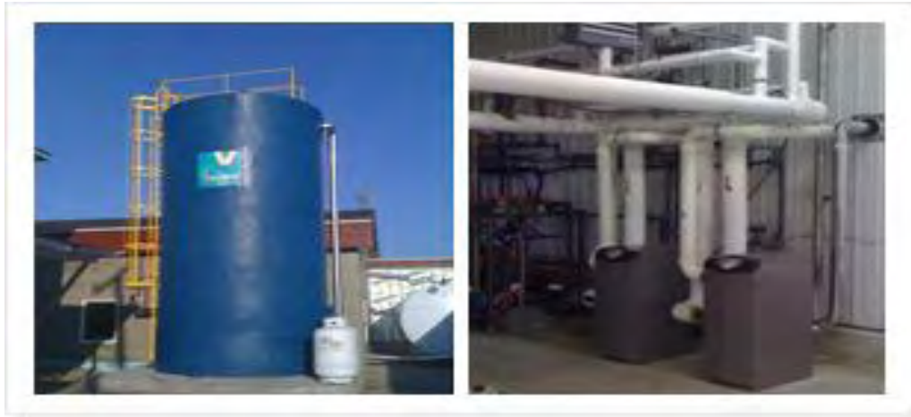
Figure 2-10 Treatment unit of anaerobic digestion of the Dairy industry La Vachea Maillotte Cheese Dairy [156].
