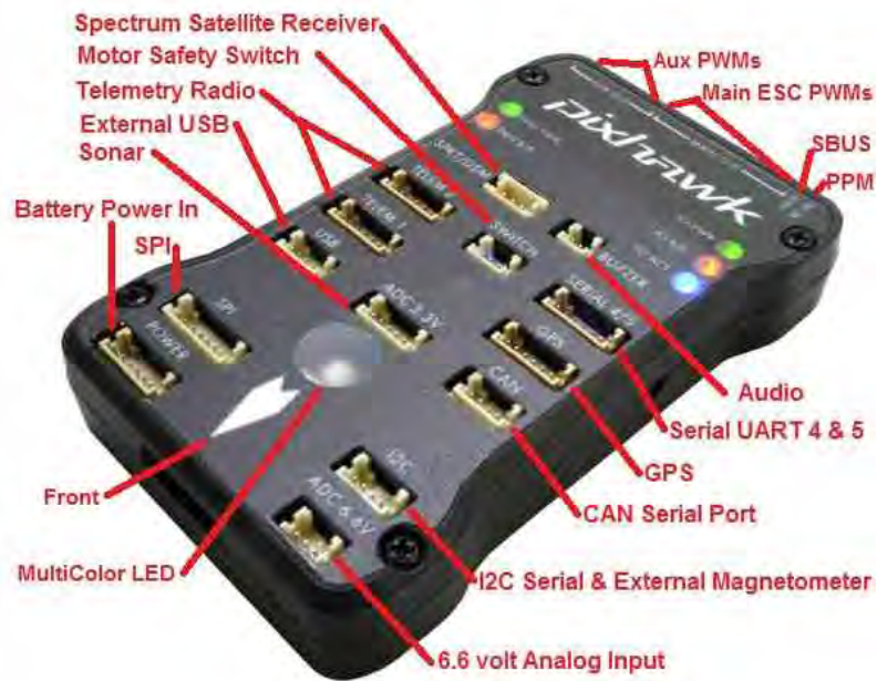
Figure 4.4: Hardware interface of the Pixhawk hardware, top
