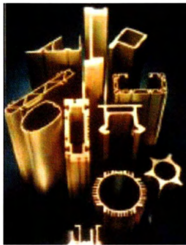
Fig. 1.6 The power of extruded Al-Mg-Si alloys is the "put the metal where you need it" flexibility that these alloys and the extrusion process provide.[2]
