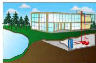
Conventional Closed Loop WSHP System
