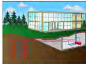
Ground-Coupled WSHP System
