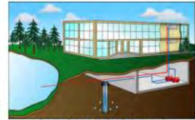
Open Loop WSHP System
