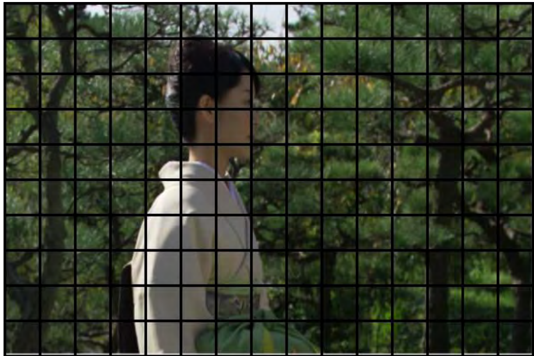
Figure 5 :A frame divided into CTUs of size 64 \times 64
