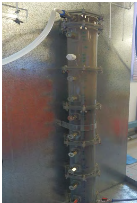
Figure 5.24 CS front at the fourth 20cm section of the 1m column of Test No8. Observe that the pipe leading to the outlet chamber shows no evidence of dye.
