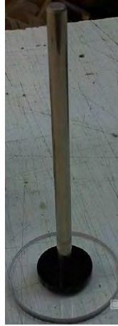
Figure 5.4 Tamper used for the compaction of soil sub-layers within the Plexiglass cylinder used for the one dimensional column injection tests.
