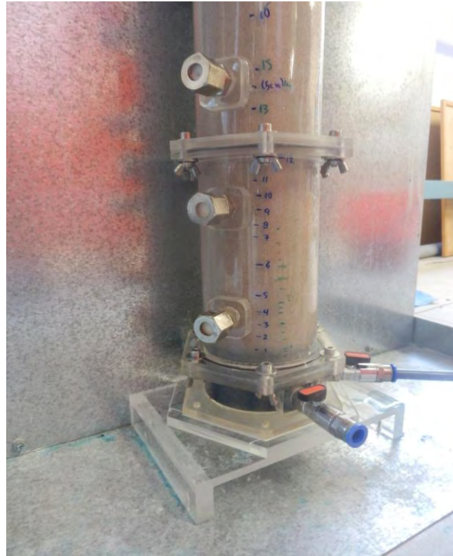
Figure 5.23 Dyed CS appears at the bottom of the sand layer at the beginning of Test No8. Observe the dyed blue pipe injecting the CS solution into the sample.
