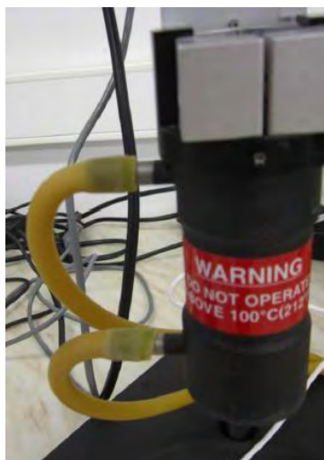
Figure 4.5 Connection of water bath to viscometer.
