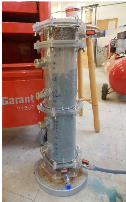
Figure 5.40. Non-uniform delivery of CS solution through sea water saturated sand column in Test No1SW.
