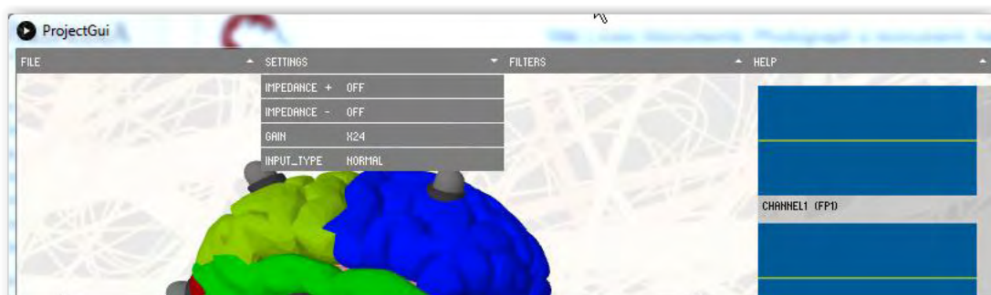
Figure 27: Settings include IMPEDANCE+, IMPEDANCE-,GAIN, INPUT_TYPE, BIAS, SRB1, SRB2
