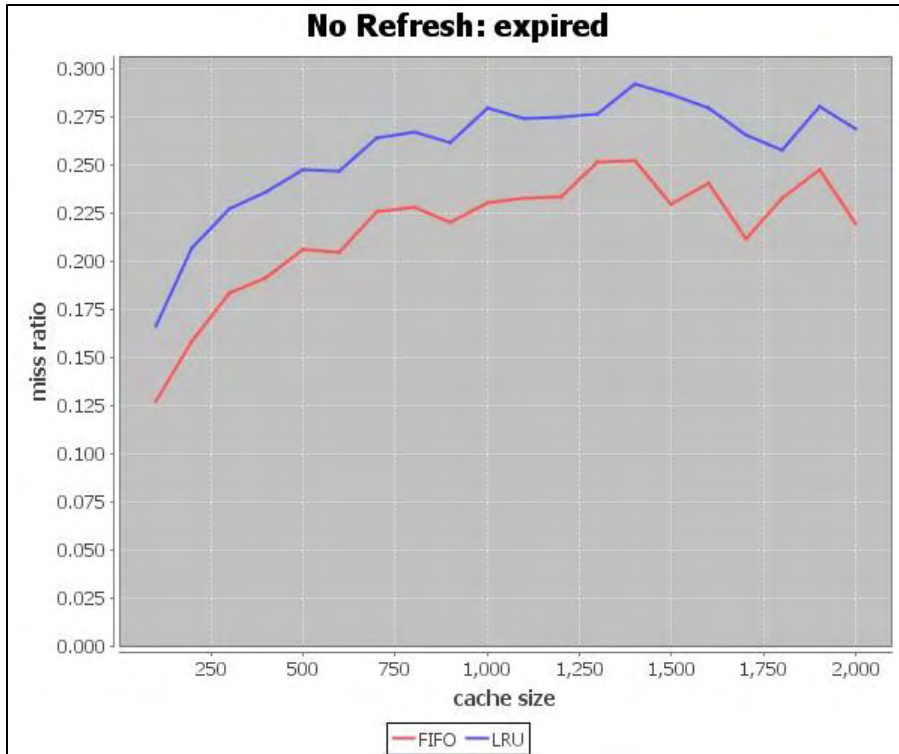
Εικόνα 18: miss ratio due to expiration (uniform TTL)
