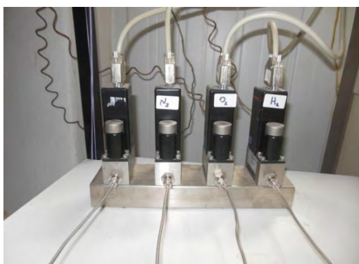
Figure 3.7. Instrumental apparatus used in the experiment with a focus on moisture saturators and mass flow meters.
