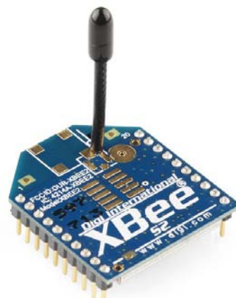
Figure 3 : Xbee S2 module for wireless communication
