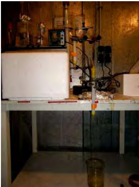
Figure 5. Cation exchange chromatography
