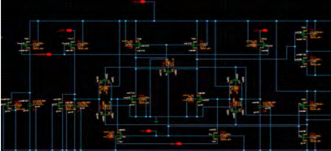
Design of Sense Amplifier circuit using Cadence Spectre tool.
