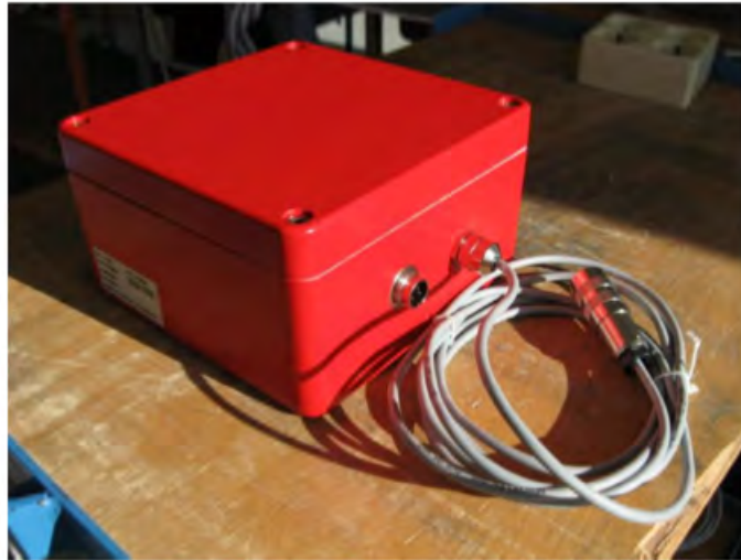
Figure 2.3: The external battery pack with integrated charger
