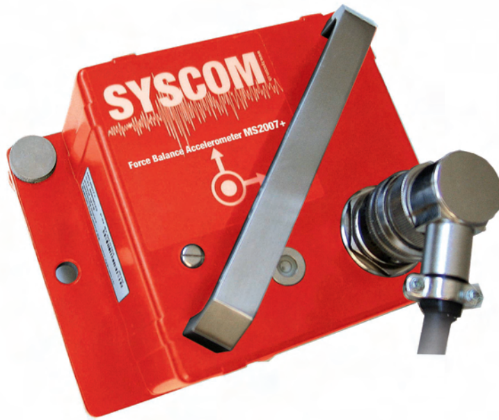
Figure 2.13: The MS2007+ Force Balance Accelerometer
