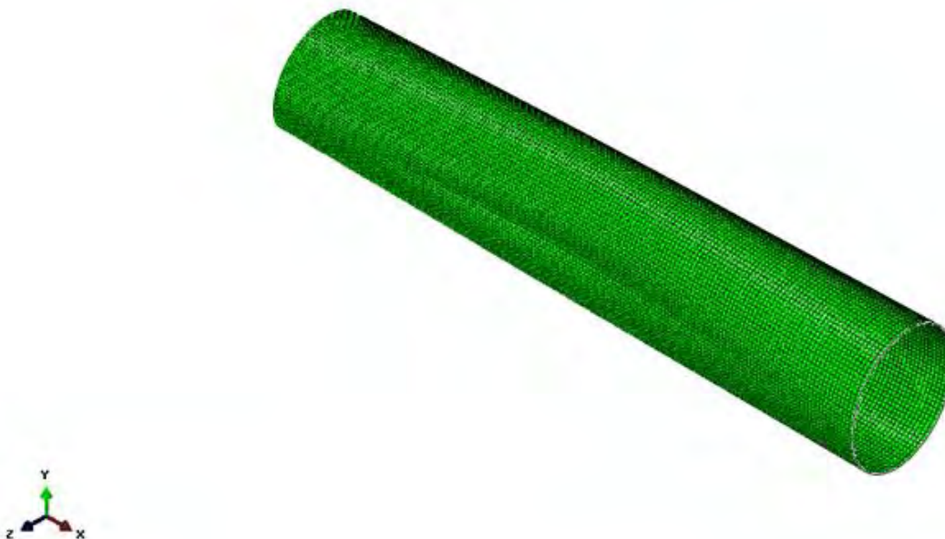
Figure 14 Post-buckling shape of specimen 9A
