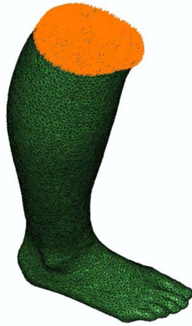
Figure 6.34: Boundary conditions applied in the present case shown in orange (fixed upper bound of the leg).
