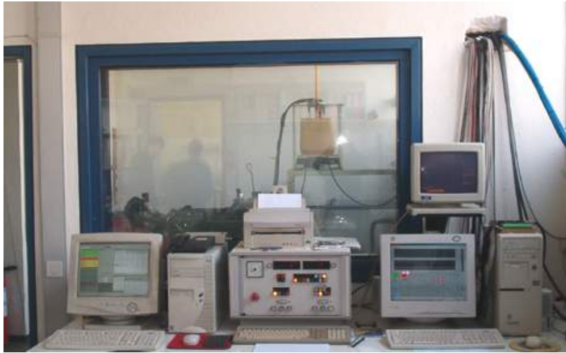
Figure 7.3 Engine and dynamometer control section
