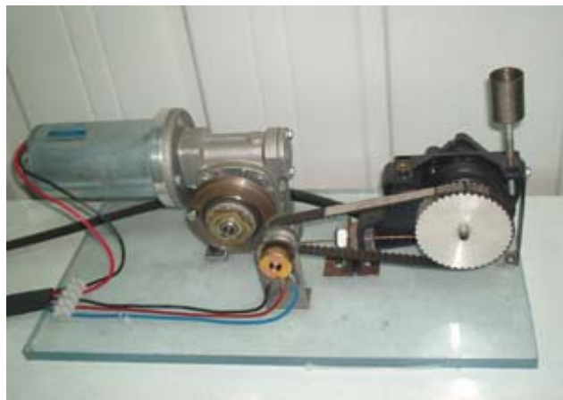
Figure 7.3 Engine and dynamometer control section
