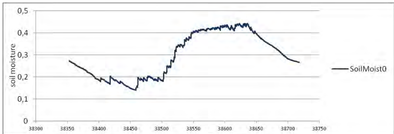
Fig. 35 Soil moisture for vertical conductivity \sim 10^{-5} and lateral conductivity equal to 0.0001 for the year 2005
