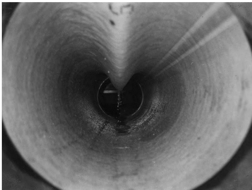
Figure 9: External pressure collapse of a confined pipe; buckling mode in the form an “inward lobe”. Experimental testing by Omara et al. [5].
