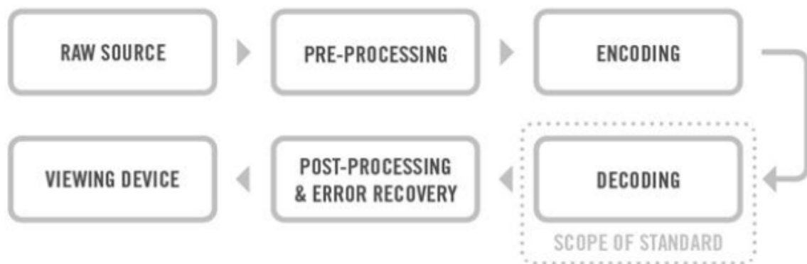
Fig. 2 Basic stages of video codecs
