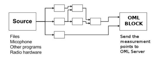
The general idea of a GNU Radio block and its structure:
