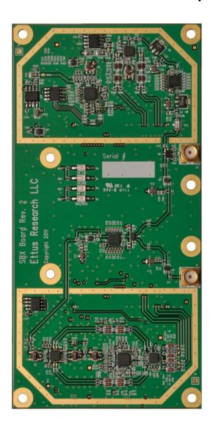
The SBX is a wide bandwidth transceiver that provides up to 100 mW of output power, and a typical noise figure of 5 dB. The local oscillators for the receive and transmit chains operate independently, which allows dualband operation. The SBX is MIMO capable, and provides 40 MHz of bandwidth. The SBX is ideal for applications requiring access to a variety of bands in the 400 MHz-4400 MHz range. Example application areas include Wi-Fi, WiMax, S-band transceivers and 2.4 GHz ISM band transceivers.
