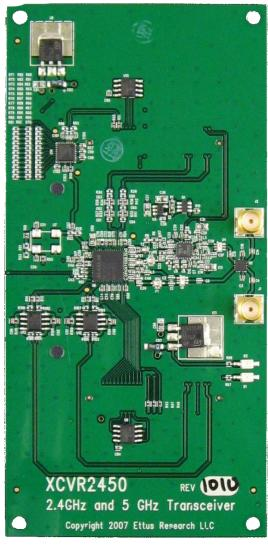
The XCVR2450 is a high-performance transceiver intended for operation 2.4 GHz and 5.9 GHz range. Filtering on the XCVR2450 provides exceptional selectivity and dynamic range in the intended bands of operation. The typical power output of the XCVR2450 is 100 mW. Example applications include public safety, UNII, ISM, Japanese wireless and UWB development platforms. The XCVR2450 is a half-duplex transceiver.
