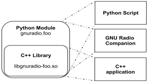
The python script initializes the blocks, connect them and send the command for execution. The GNU Radio Companion part is an XML file that represent the block in the graphical tool. In the C++ application the signal processing is taking place.
