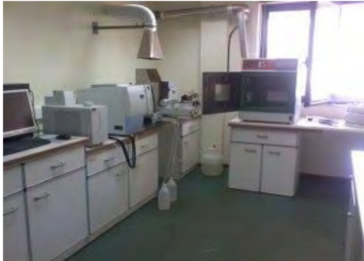
Εικόνα 2.4: Microwave 3000, Sample Preparation System, Anton Paar, Microwave Reaction System Perkin Elmer
