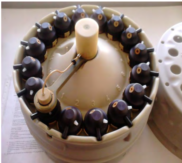
Εικόνα 2.5: Microwave 3000, Sample Preparation System, Anton Paar, Microwave Reaction System Perkin Elmer
