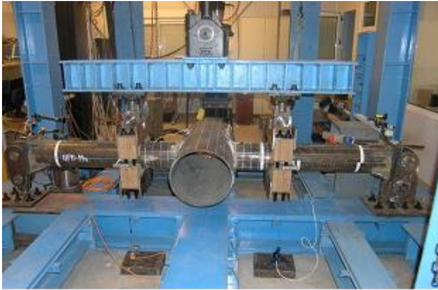
Figure 5.3: Test configuration for OPB loading.
