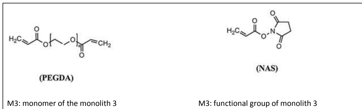
Fig5. Chemical structures of the NAS which is the active monomer for M3 (functional group) and offers high activity to react with the amino group of the enzymes and the PEGDA used as the cross-linker.
