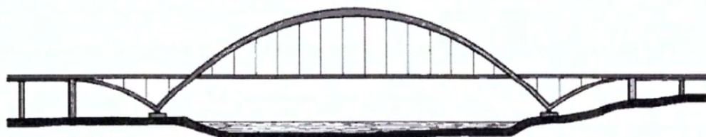
Arch bridge with cantilevering side span arches.
