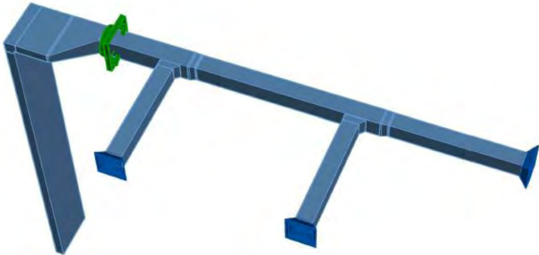
Figure 3-7 Typical connection of fan and takeoffs for space heating to the main duct receiving heated air from one of the 8 ducts behind a band of 6 PV modules.
