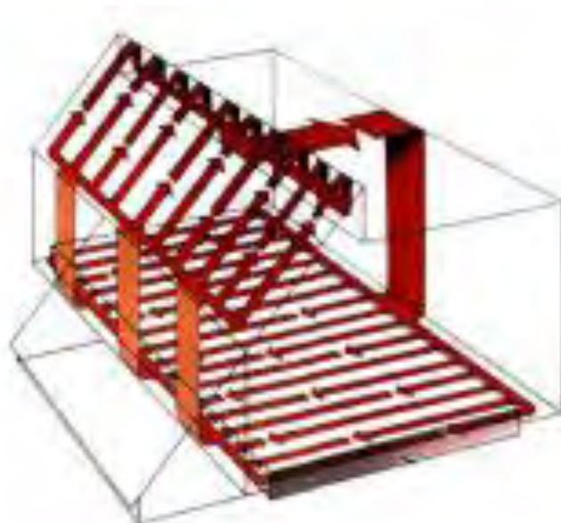
Figure 2-2 The hybrid collector provides warm air to the heating system in the house of future
