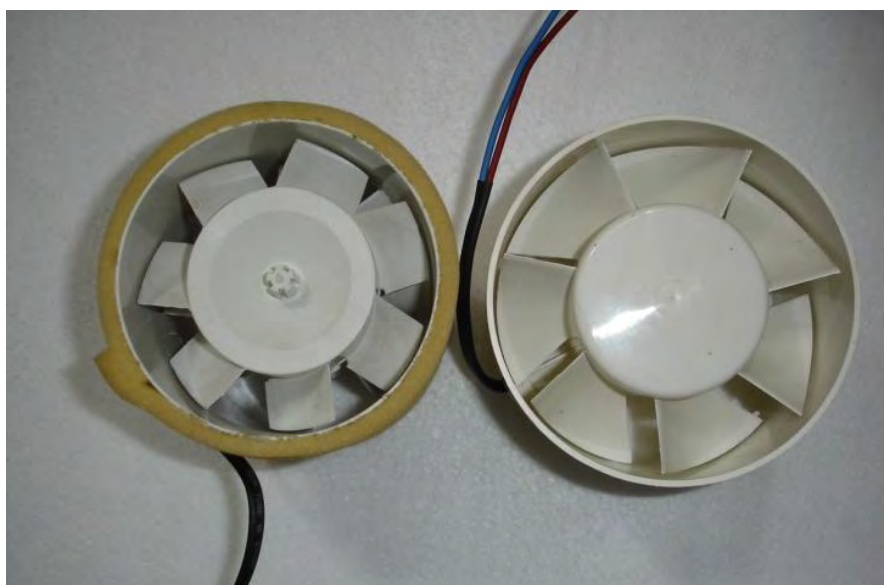
Figure 4-9 Photo of the lower and higher capacity axial fans fitted to the exit duct (20 W each).
