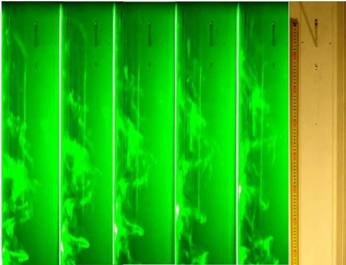
Figure 4-36 Forced convection, 190 \text{ m}^3/\text{h} fan, camera in the upper position, laser light sheet close to the right-hand frame (scale shown by the measuring tape to the right), (Video 11314, ANNEX III)
