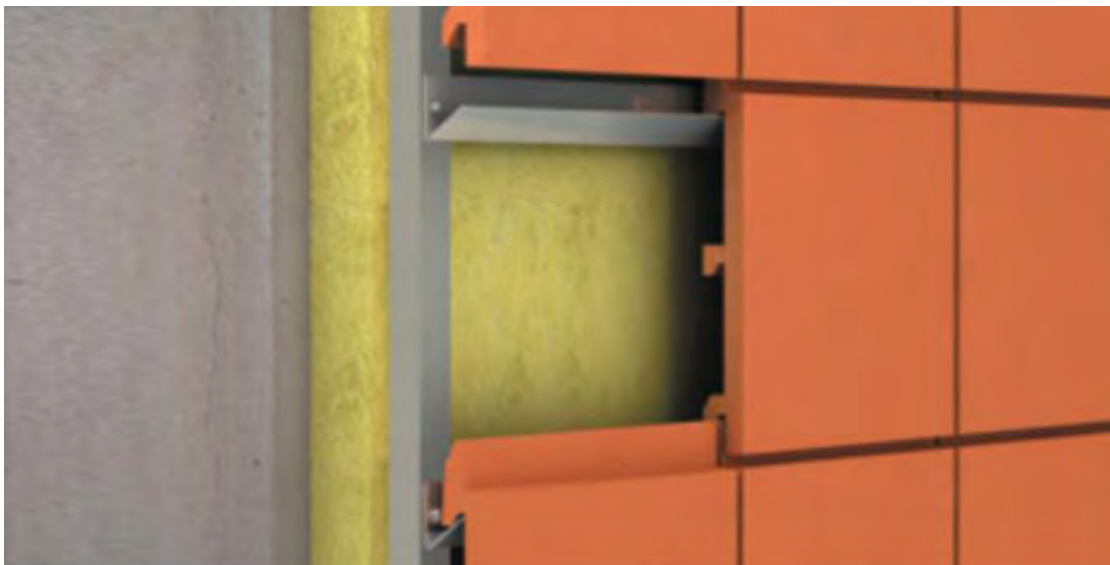
Figure 3-2 The facing tile is a single-skin cladding product which is easy and economical to install, with a lightweight system resting on horizontal rails (adapted from [135]).
