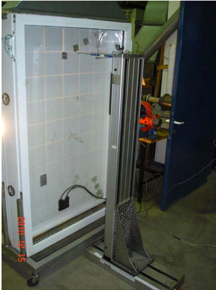
Figure 4-43 Hot wire anemometry: experimental layout
