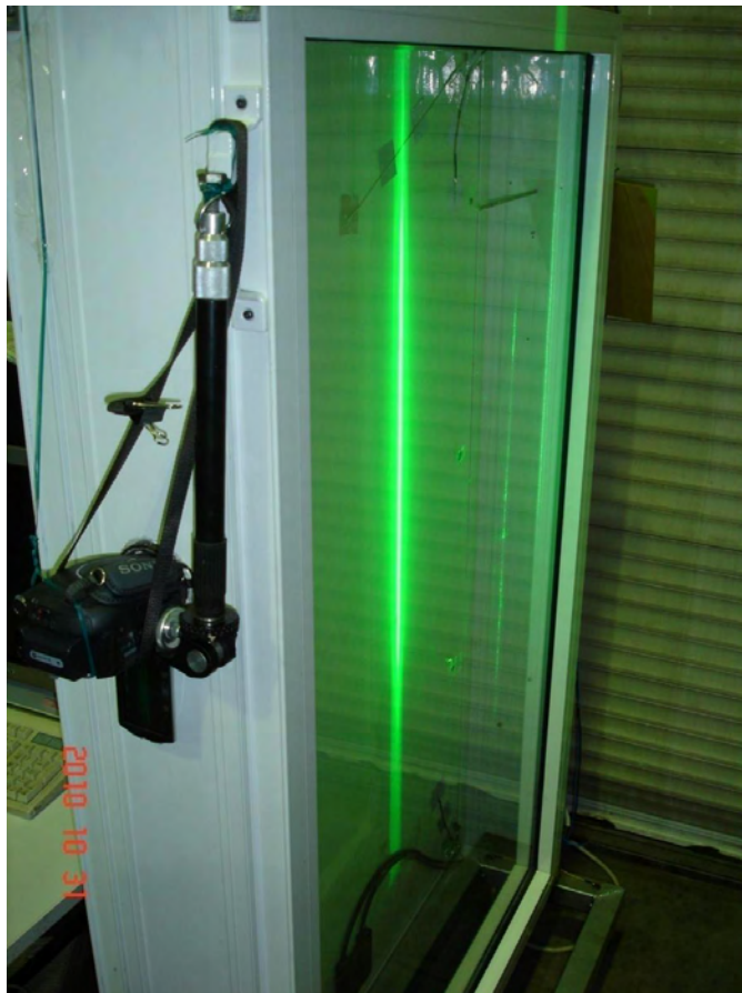
Figure 4-30 Flow visualization: experimental layout. Video-camera placed in the upper position, seeing towards laser light sheet. The honey comb flow homogenization structure has been removed in this photo.
