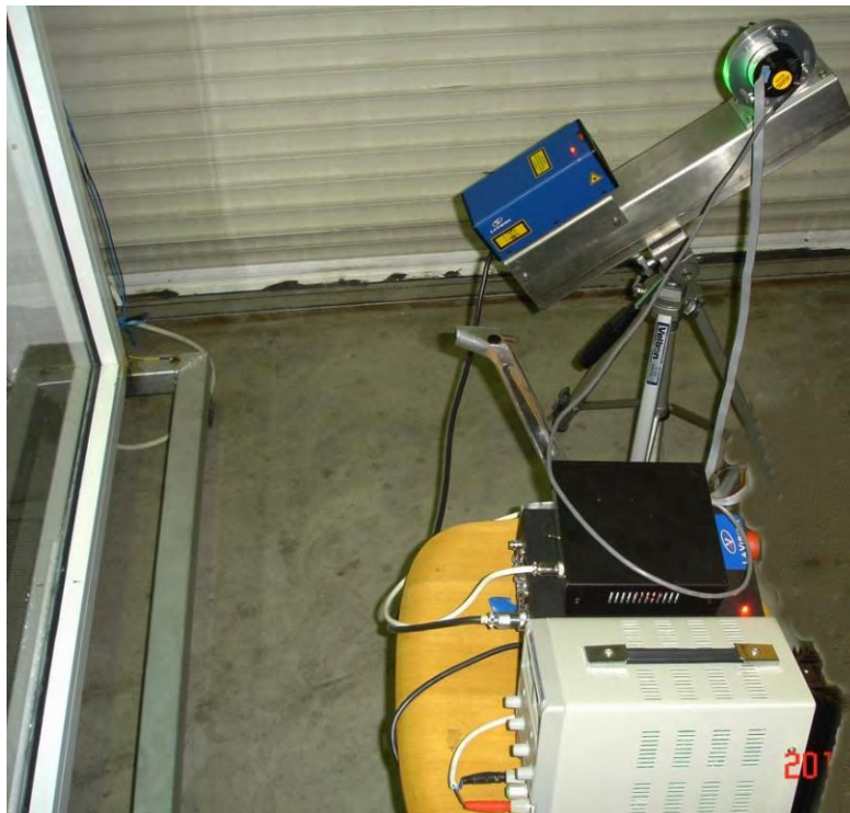
Figure 4-27 The green 1.277 W laser with the rotating mirror, power supply -control unit
