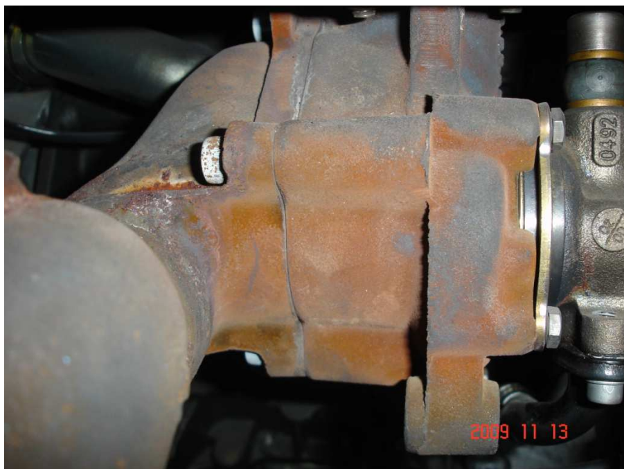
Figure 48 Turbine housing and exhaust downpipe
