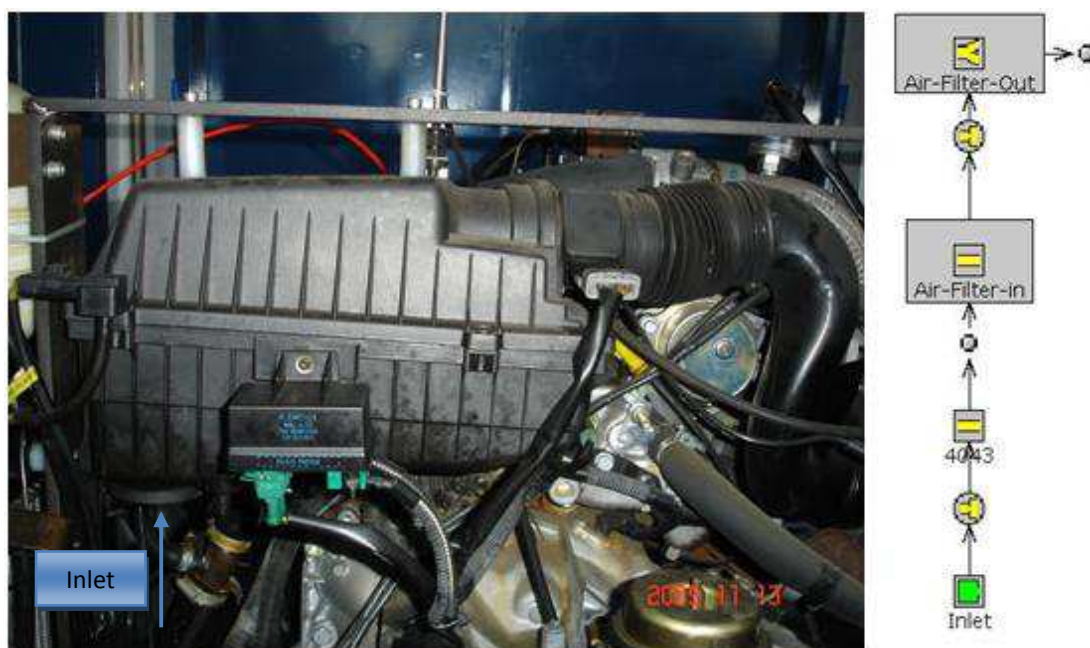
Figure 34 DW10 air box on the left and air box model on the right
