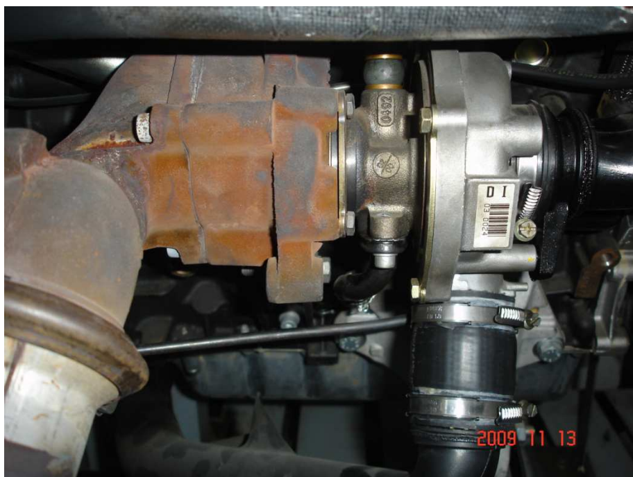
Figure 50 PSA turbocharger kit – turbine, compressor, exhaust downpipe and inlet-outlet hoses
