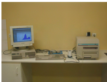
Figure 4.4: TLD reader and computer system
