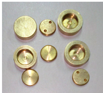
Figure 5.4. Copper build up caps for 6 and 15 MV.
