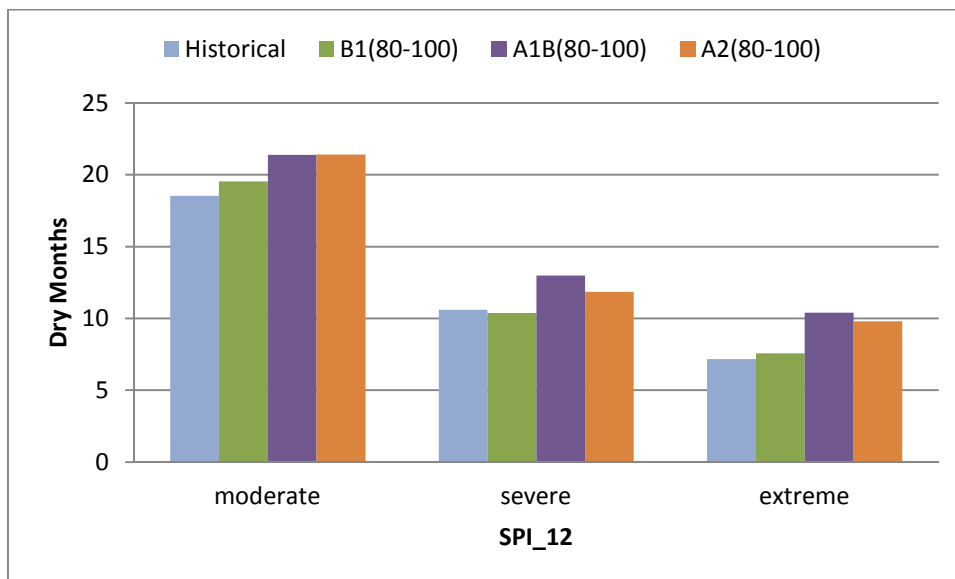
Figure 4.14. Total numbers of dry months ( SPI \leq -1 ) for various drought severity classes at 12-months timescale for the three SRES scenarios and for period 2080-2100.
