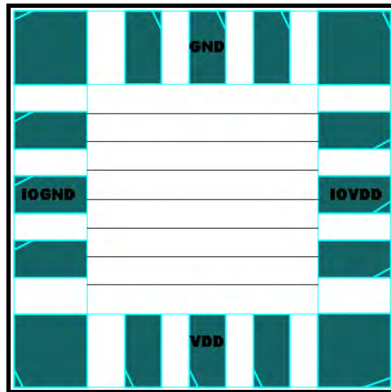
ΕΙΚΟΝΑ 3.7: I/O, PWR/GND, Corner PAD placement
