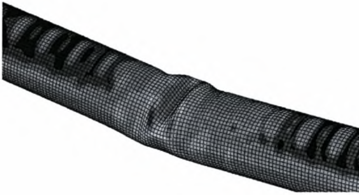
Figure 6.3.3b Deformed geometry of the tube model with D=323.9\text{mm} , t=10\text{mm} and L=3\text{m} ( w_0=0.5t ) under axial compression up to 0.5N_a and bending.
