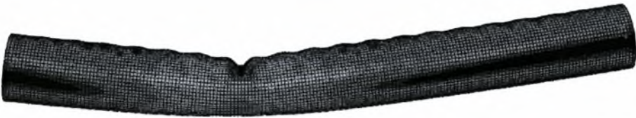
Figure 6.3.3c Deformed geometry of the tube model with D=323.9\text{mm} , t=10\text{mm} and L=3\text{m} ( w_0=0.5t ) under pure bending
