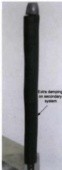
Figure 5.24: TMD with insulation material for extra damping
