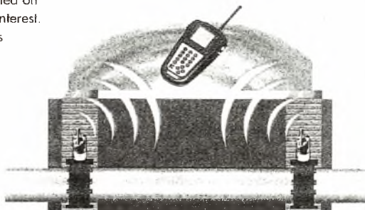
Permalog® units transmit leak status signals to the Patroller.
