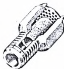
Breather assembly with surfactant-treated porous element
